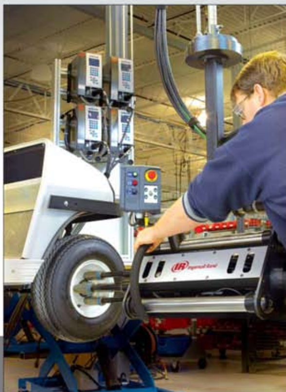
4-spindle horizontal/rotative DC fastening system
