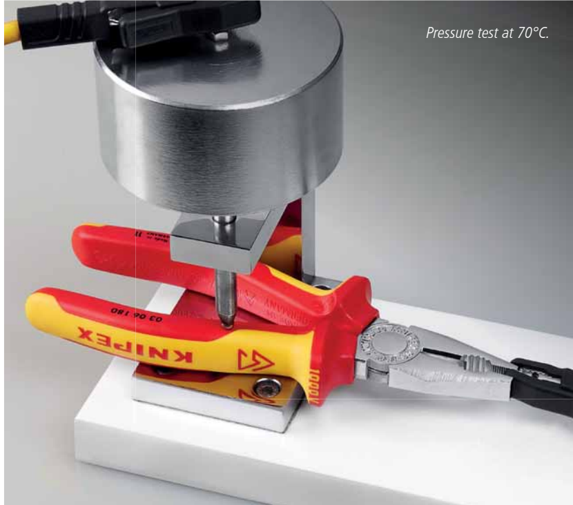
Testing dielectric strength, subjecting each pair of pliers to a load of 10,000 V AC.
