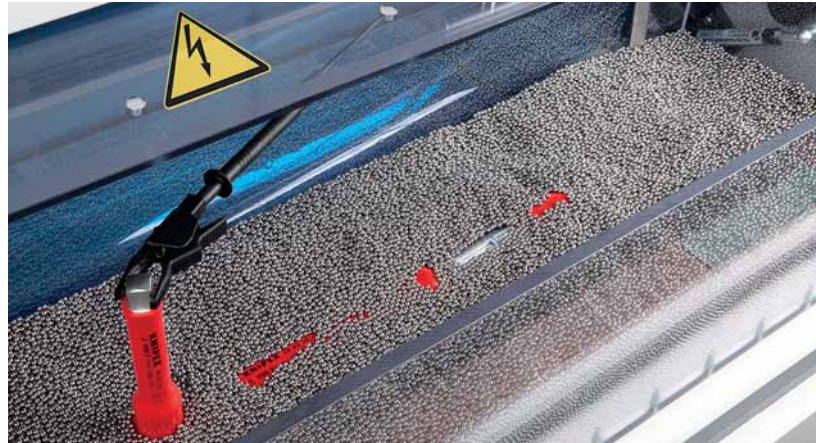
Testing the electrical insulating properties.
