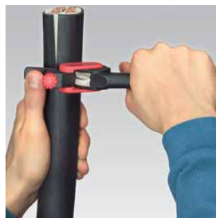
Turning the tool for circumferential cut
