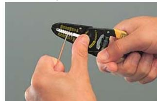
For cutting and stripping of various electronic wires represented by KV
