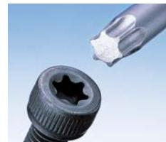
Basic TORX consists of 6 ear-lobular shaped curves. Compared to hexagonal shape driver, TORX has higher drive effectiveness and transfers torque smoothly and accurately while eliminating "CAM-OUT".
