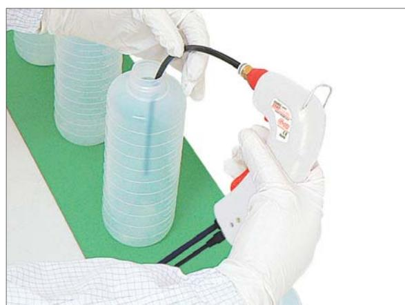
Static electricity removal in a bottle
