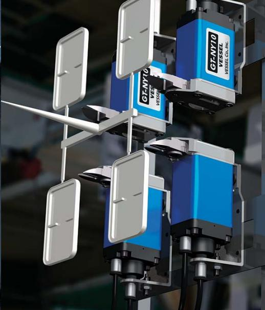
These are high-class air nippers that can be mounted on gate cutting equipment and standby jigs for accurate, speedy cutting of resin products. VESSEL has a wide selection of items to meet a variety of needs not only for around-the-clock operations but also for the highly precise cutting accuracy.
