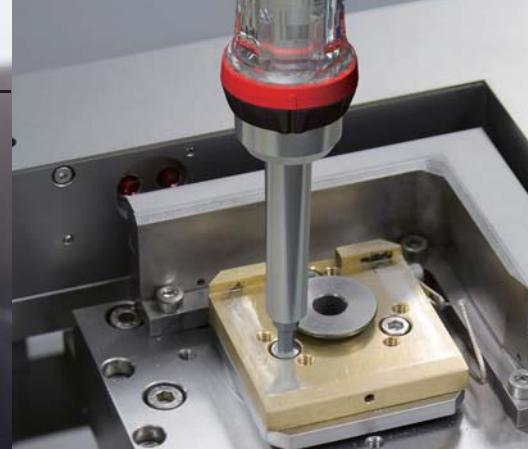
This functionally enhanced screwdriver enables screw tightening by simple repeated wrist movements.
