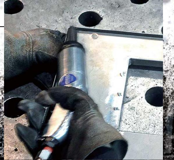
The barycenter is at the front side, alleviating the strain on your wrist. Effortless operation is possible by just pressing the needles on welding spatters, slugs, etc. The impact does not catch your hand so the needles do not spread out as much, making it easier to work.
