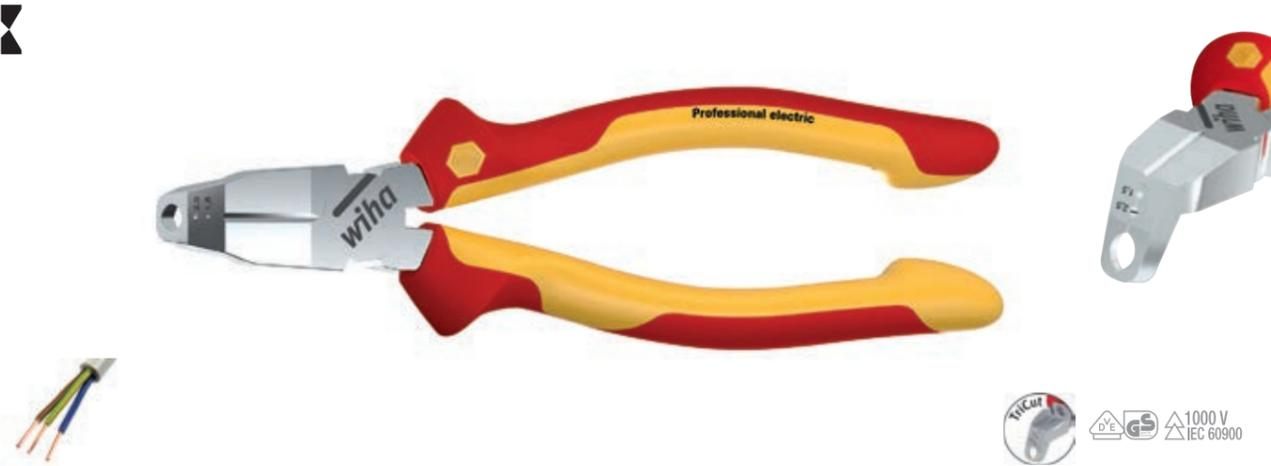
**Simplifies your work:** The angled head allows you to work in hard-to-reach places such as installation sockets. **Lowers your costs:** Now you only need one tool for three tasks: cutting to length, stripping and skinning. **Increases your efficiency:** Three tools in one. Saves 60% volume and 50% less weight for 100% efficiency. **Offers you full protection:** Each tool individually tested at 10,000 V AC and approved for 1,000 V AC.
